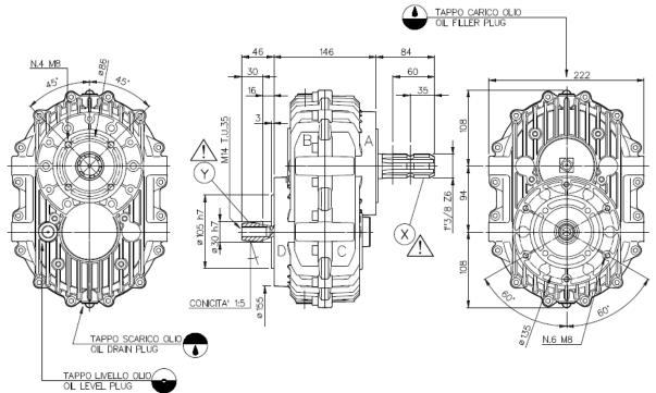
Check Oil every 8 hrs: Oil level is correct if the lower edge of the inspection hole is nearly covered with oil. \*\*If your gearbox differs from the one above, contact IMD.
